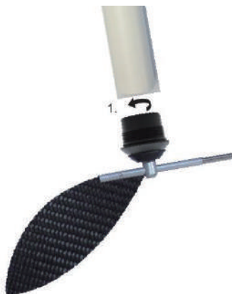
Figure 9.( Bearing replacement – Wind speed/direction sensor)
